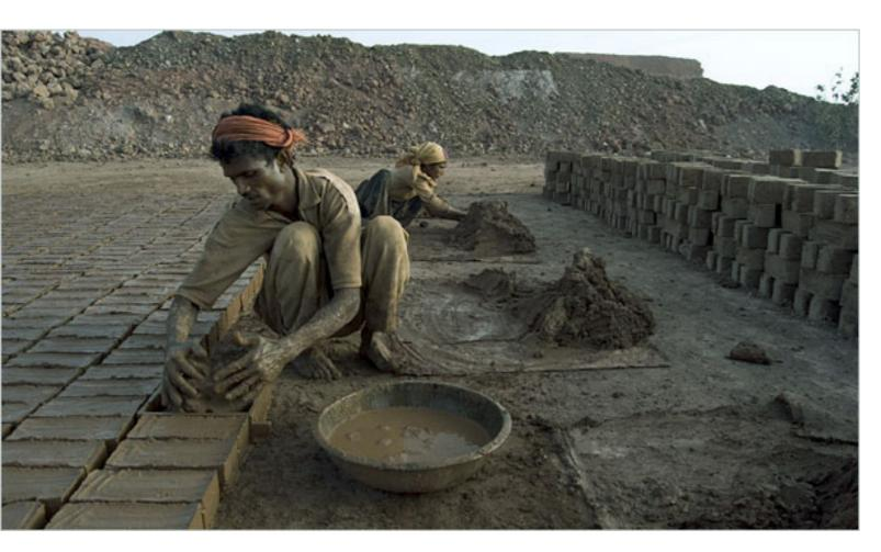
Bricks are one of the oldest known building materials devised by humans; their first appearance dates back to the nearly 7000BC. Naturally, the methods for their manufacture have improved tremendously over time, transitioning from the hand shaping and moulding to todays mechanised, high-volume mass produced extrusion systems. Yet despite the advancements in the manufacturating methodology and exploration in configuration, the overall geometry of the brick itself has changed very little.
